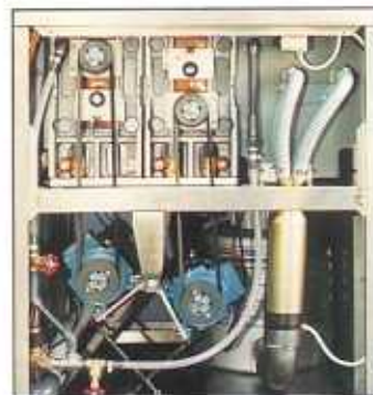
Photo (at left) shows internal view of the rear of a CDO/DH showing the brush drive system, plumbing for the rinse jets and the high capacity blower delivering heated air to the airknives via flexible hose.
