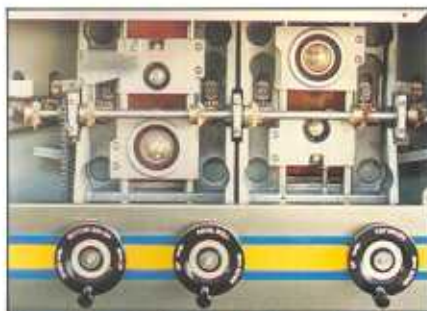
Photo (above) showing brush and anvil bearings mounted in heavy duty anodised aluminium castings, supported by precision ground stainless steel slideways. Also shown is the conveyor nip roller drive system incorporating heavy duty bevel gears.
