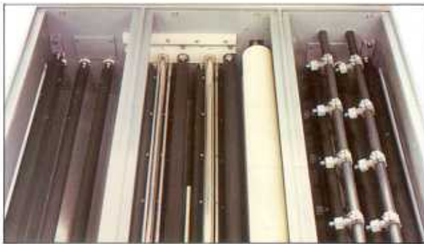
Shown above is central compartment of HSRD showing 2 pairs of spray tubes in the rinse section followed by a pair of squeegee rollers and 2 pairs of airknives mounted in self-adjusting carriers in the drying section.
