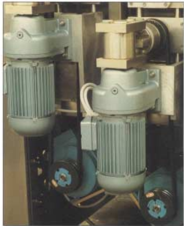
The photo of the rear of the machine (above) shows the brush rotation motors, oscillation motors, oscillating drive mechanism and rear bearing housings.
